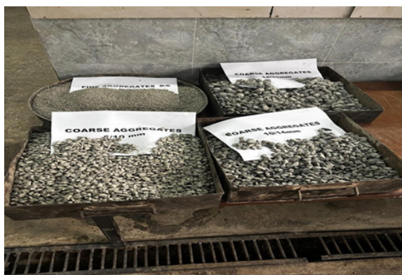
Nominal representative sample aggregates used in the HMA mix designs
