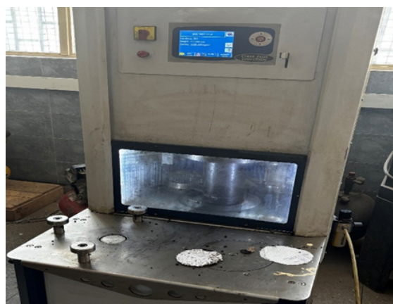
SUPERPAVE Gyratory Compactor equipment used in the SUPERPAVE compaction test
