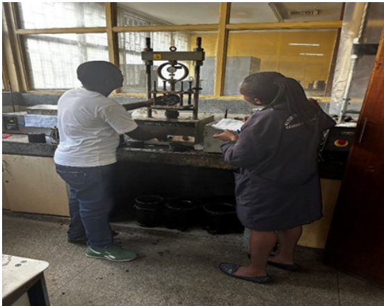
Ongoing test for Indirect tensile strength and dial gauge reading
