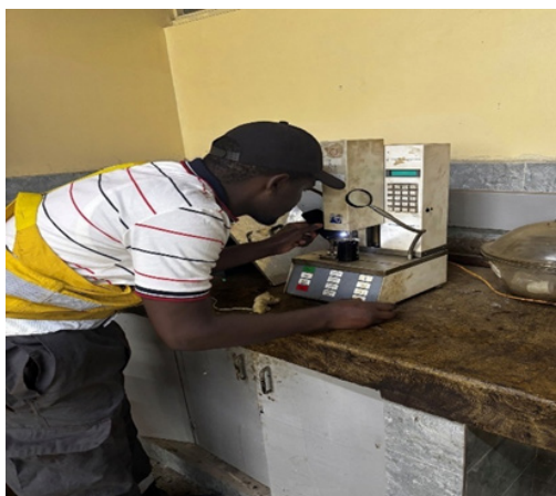
Evaluation of bitumen binder using penetration test at 25 °C
