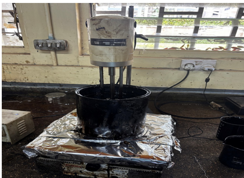
FIGURE 3 Mixing of 60/70 penetration grade bitumen and SBS using High-Shear Mixer Source: Field survey, 2025
