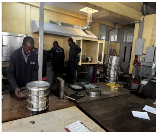
Sieve analysis for crushed limestone aggregates
