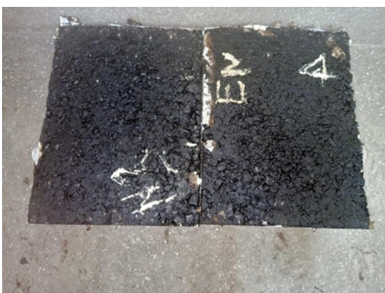
Compacted neat HMA in a rectangular slab ready to be mounted on a double-wheel tracker for a rut depth test
