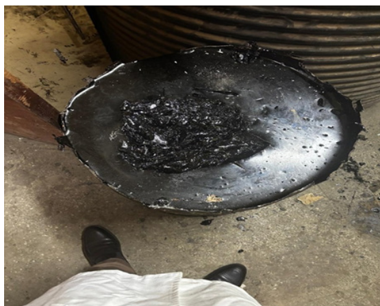
A drum of 60/70 penetration grade bitumen sample used in the mix designs
