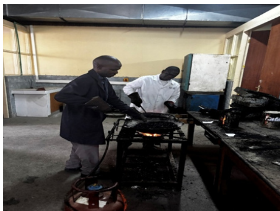
Manual pre-heating and mixing of measured aggregates and 60/70 penetration grade bitumen
