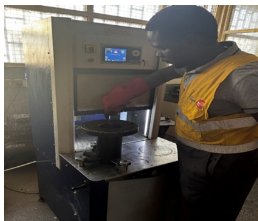
Setting up of HMA sample into the SUPERPAVE Gyratory mould
