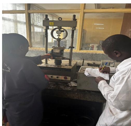
Ongoing test for Marshall stability and dial gauge reading
