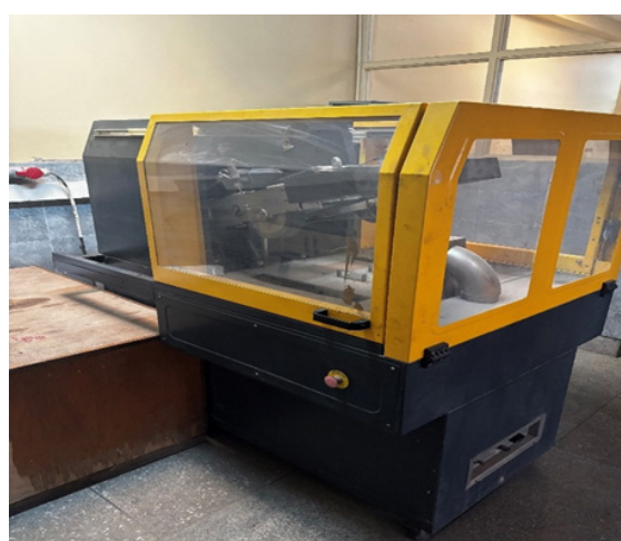
Double wheel tracker (EN12697-22) used in the Rut depth test
