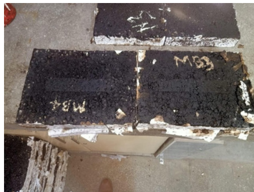
Compacted modified HMA in a rectangular slab, ready to be mounted on a double-wheel tracker for a rut depth test
